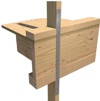
Rolled Strap Installation
