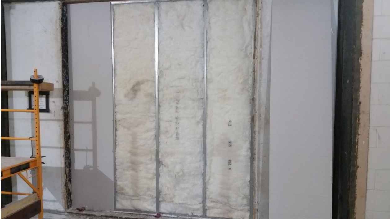
Figure 7 – Insulation installed in stud cavities, receive room side partially installed, viewed from receive room
