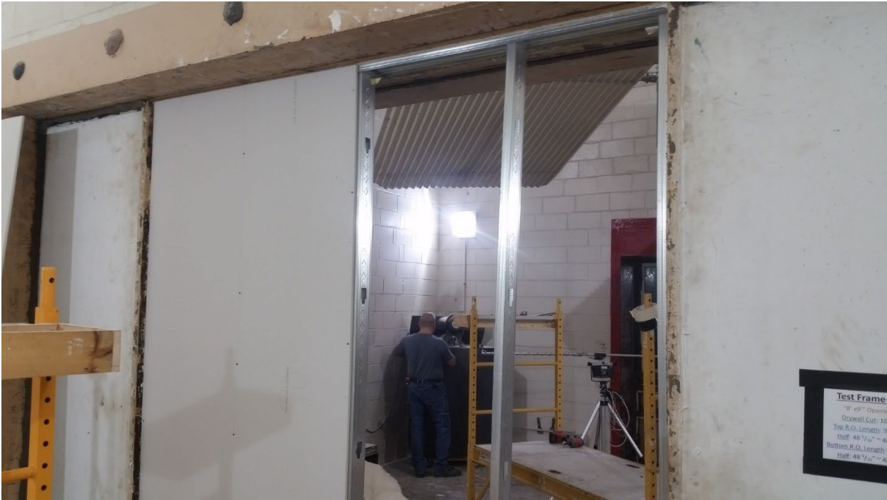
Figure 3 – Tracks and studs installed in test aperture, source side gypsum board partially installed
