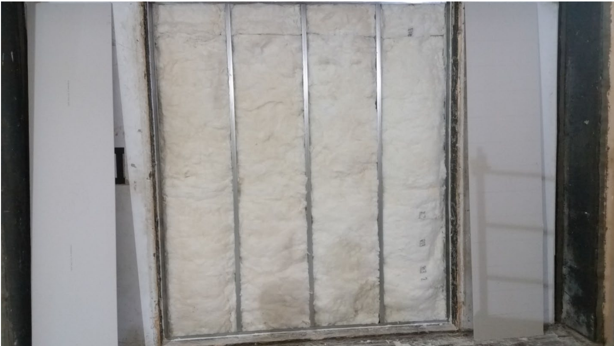
Figure 6 – Insulation installed in stud cavities, viewed from receive room
