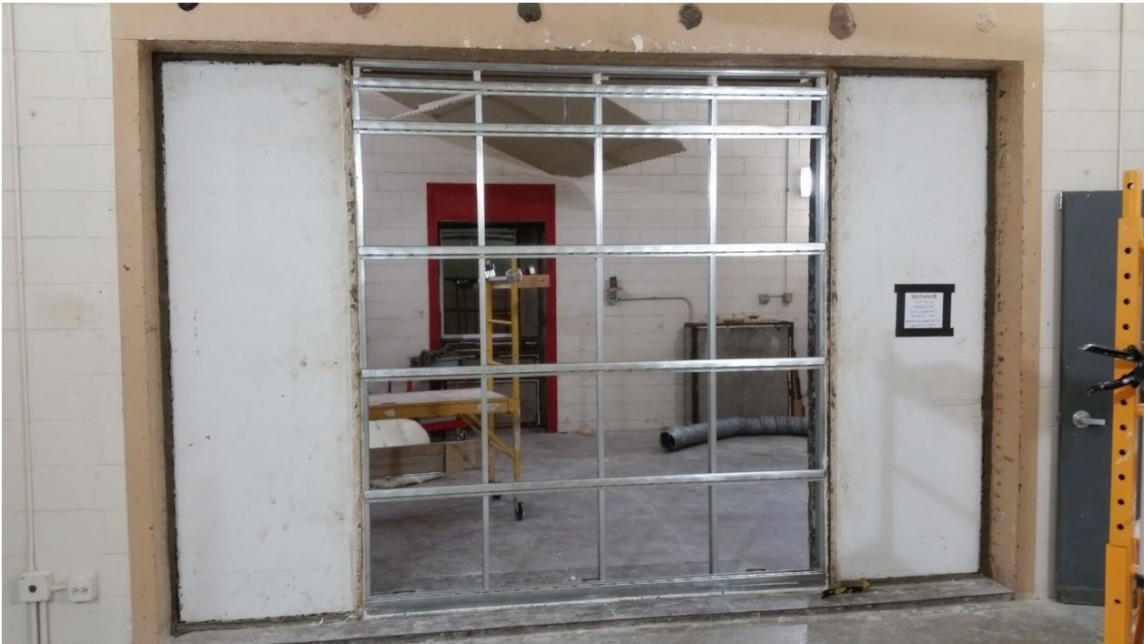
Figure 4 – Tracks, studs, ProStud Motion Frame Connectors, and resilient channel installed in test aperture
