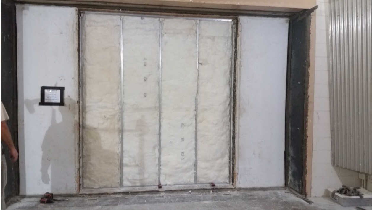
Figure 9 – Insulation installed in stud cavities, viewed from receive room
