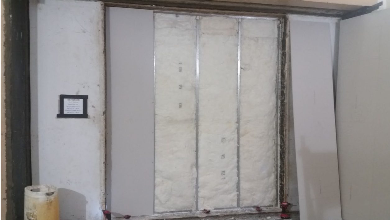
Figure 11 – Receive side base layer gypsum board partially installed
