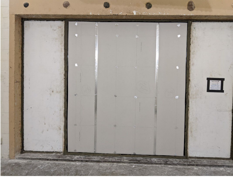
Figure 1 – Specimen mounted in test aperture, as viewed from source room
