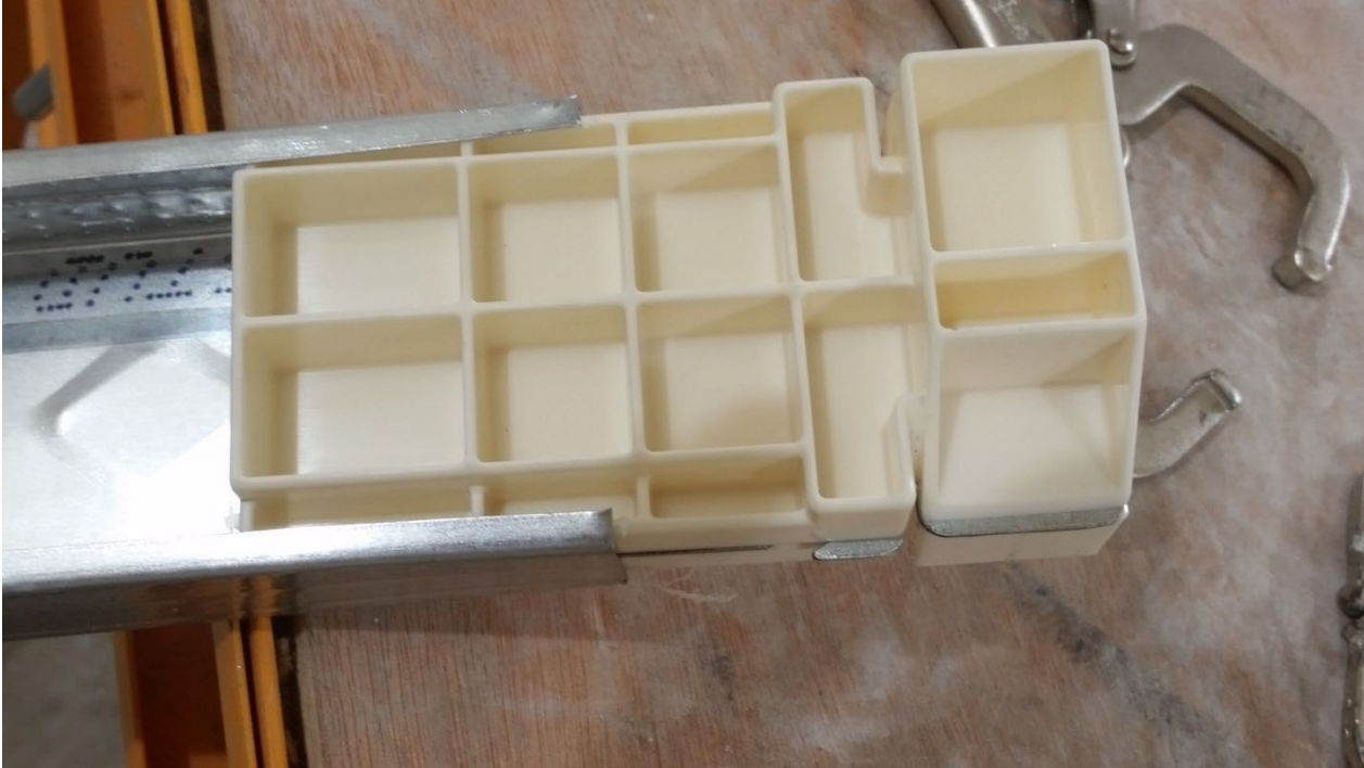
Figure 3 – Stud with ProStud Motion Frame Connector attached, prior to installation in test aperture
