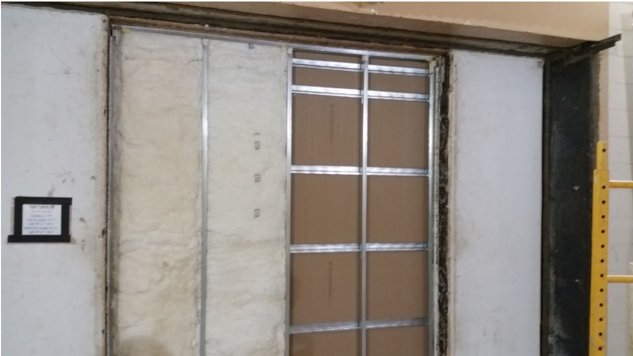
Figure 8 – Insulation partially installed in stud cavities, viewed from receive room
