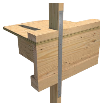
Rolled Strap Installation
