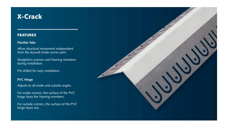
**NO CRACKS** X-Crack® eliminates all cracks in vaulted ceilings, butterfly vaults, and inside 90-degree corners in flat ceiling areas caused by truss uplifts. This patented product holds drywall joints stationary while allowing structural movement of framing members.
