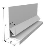
Designed for wall transitions where a brick or stone ledge is involved. Positive drain ground leg tilted at 45° so that water can run off with a secondary leg to push water away from wall.
