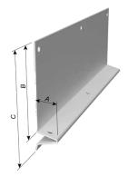
The traditional style. It is designed to relieve moisture from the wall and act as a stop. Install on frame construction where stone veneer and foundation meet.
