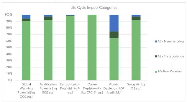
The weighted average cradle-to-gate GWP of ClarkDietrich's cold-formed steel products across all sites is 1,659 kg CO<sub>2</sub>e/metric ton, about 25% lower than the GSA limit for cold-formed and galvanized steel products at 2,228 kg CO<sub>2</sub>e/metric ton. The cradle-to-gate GWP for each individual site also falls below the GSA.
