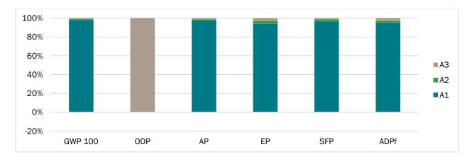
For most impact categories/indicators, the production of raw material inputs accounts for most of the impacts, which is mainly attributed to the steel coil used to create the framing products.
