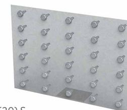
(30) Screws (18) at Header (12) at Jamb
