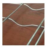
Designed to promote uniform plaster thickness and provide superior reinforcement and crack resistance. The longitudinal wires are cold rolled (flattened) to eliminate curvature memory. The hat channel furr provides superior stucco embedment and each and every cross wire is securely furred.
