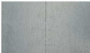
Surface rust 240 hours DIAMONDPLUS: 1.00%
