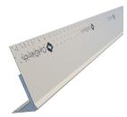
L-trims are used to finish the ends of wallboard where it abuts dissimilar surfaces, such as suspended ceilings, beams, plaster, masonry or untrimmed door and window jambs. Applied in the same manner as all other tape-on beads-joint compound embeds the paper-faced bead to the wallboard paper.
