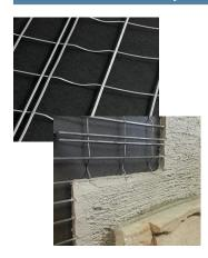
Welded wire lath produced according to ASTM C933 by Structa Wire Corp. and distributed by ClarkDietrich. Comes in rolls, not sheets. Goes up fast, lays flat, simple to install.
