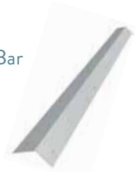
The TradeReady® SPAZZER® 5400 bar provides bridging for structural stud systems without mechanical attachment (Except in axial load bearing applications) in much the same way the SPAZZER 9200 bar works for drywall partitions. The 5400 is galvanized 16-gauge bar that is 50" long and is notched to rigidly hold studs on 12", 16" or 24" centers.
