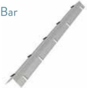
The TradeReady® SPAZZER® 9200 bar provides bridging for drywall stud systems without mechanical attachment. The 9200 is a 20-gauge bar that is 50" long and is pre-notched to rigidly hold studs on 12", 16" and 24" centers. A new concept in bridging, the 9200 bar is simply passed through the stud punch-outs, rotated 90 degrees, and then the pre-notched slots are seated down over the web of the stud.
