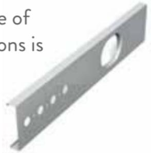
The uniquely designed TradeReady® Joist Rim drastically reduces framing layout by providing pre-punched tabs at either 12, 16, 19.2 or 24 inch o.c. The pre-cut structural blocking easily installs to the underside of the joists to prevent rotation.
