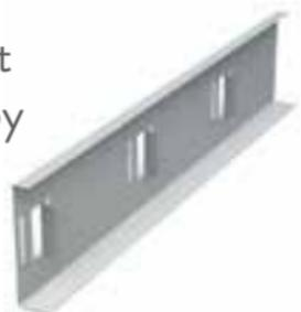
The TradeReady® System is available in a variety of sizes and thicknesses from 18-12 gauge 7-1/4" – 14" deep web members and the joist can single span in excess of 33 feet. Hole sizes range from 4-1/4" x 7", 6-1/4" x 9", 8" or 10" round based on web member size.
