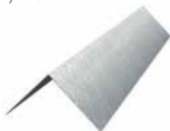
Applications: Metal Angle is made of 25 and 20 gauge, galvanized steel. All-purpose metal angle is available in three common sizes. The 1-3/8" x 7/8" size is used to secure core board to floors and ceilings in laminated drywall and veneer plaster systems. Other sizes are used for a variety of purposes.
