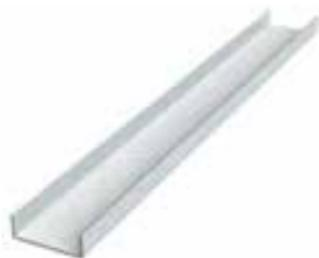
Applications: Used to laterally brace studs or with furring channels in ceiling applications. When used as lateral bracing, a clip angle is attached to both the stud and U-Channel to prevent stud rotation.
