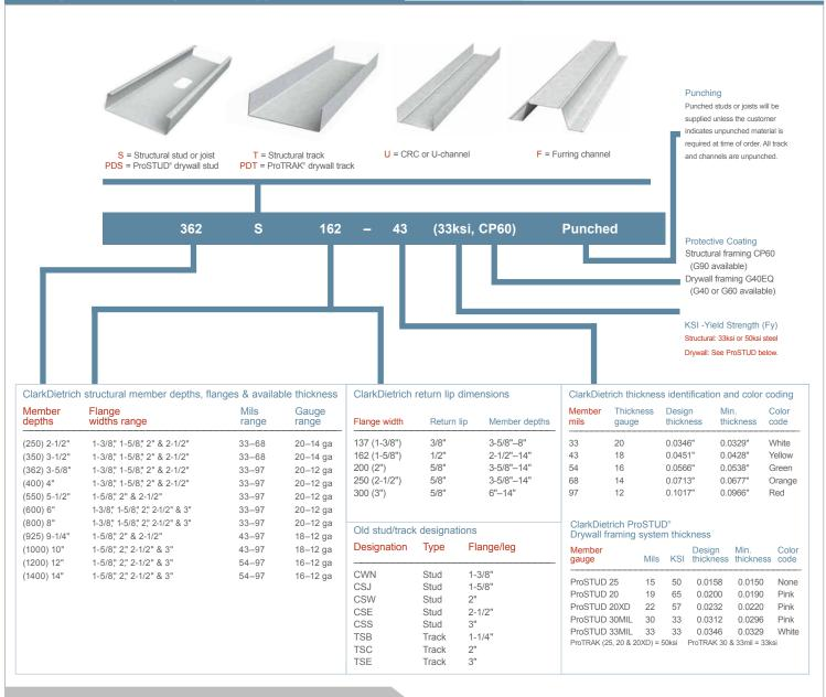
ClarkDietrich has adopted standard nomenclature established by the American Iron and Steel Institute (AISI) for identifying each of its products. Coding of each member consists of four parts, in this order:
