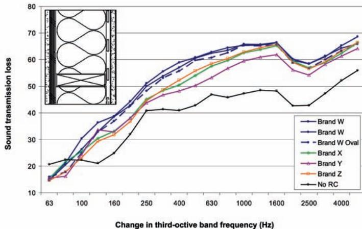
Transmission loss testing.<sup>1</sup>
