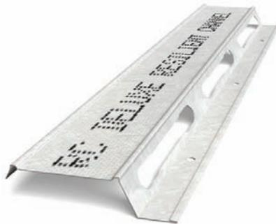
Traditional resilient channels that follow the original design typically feature a long, slotted hole with circular ends wider than the middle portion of the slot. These holes are commonly referred to as a 'dog bones.' They are 76 mm (3 in.) long and nominally 9.5 mm (3/8 in.) wide in the center; dog bones are spaced 102 mm (4 in.) on center (oc) along the sloping side of the resilient channel.
