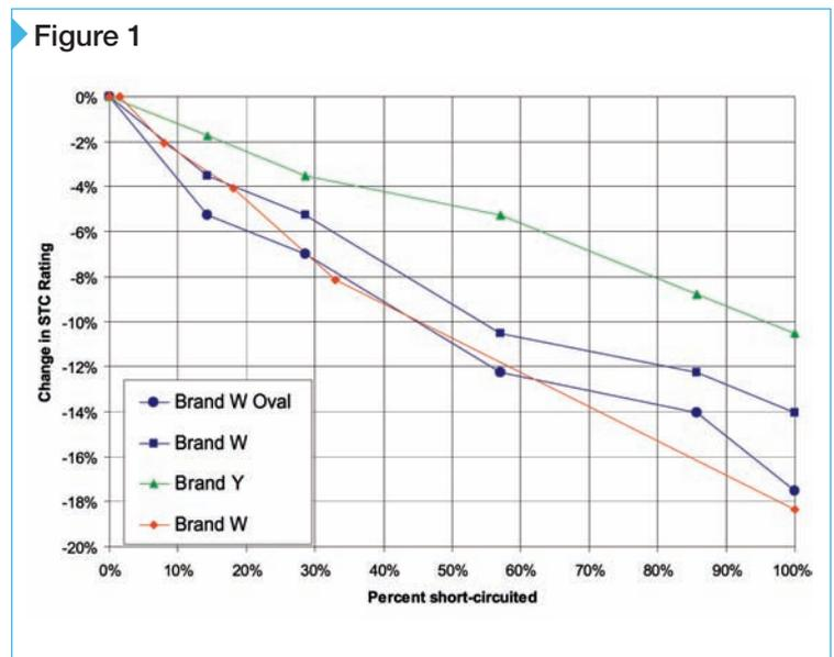
The effects of short-circuiting on a wall assembly’s sound transmission loss.<sup>1</sup>
