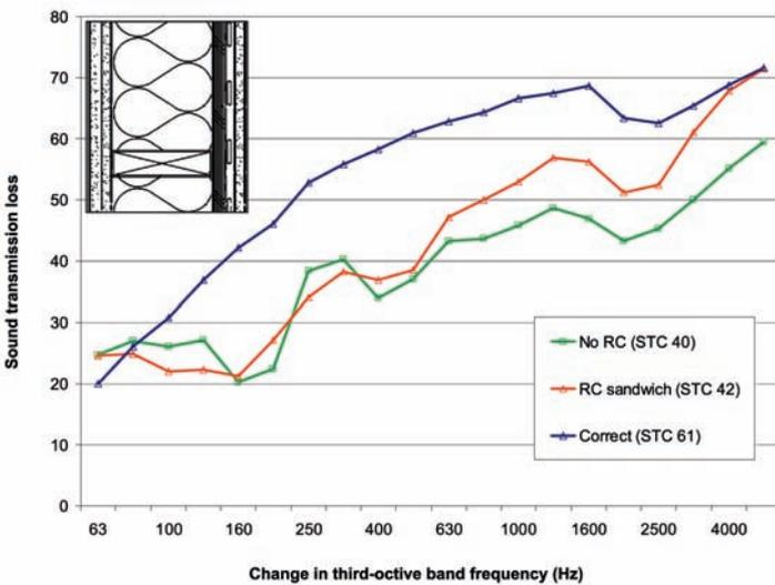
Sound transmission loss when the resilient channel is sandwiched between plywood and gypsum board in the wall assembly.<sup>1</sup>
