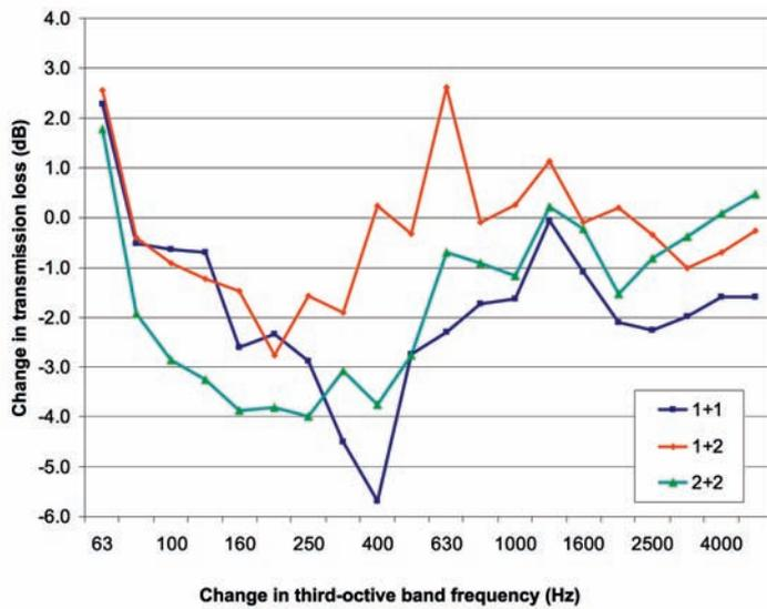
Sound transmission problems were caused by improper placement of the resilient channels.<sup>1</sup>
