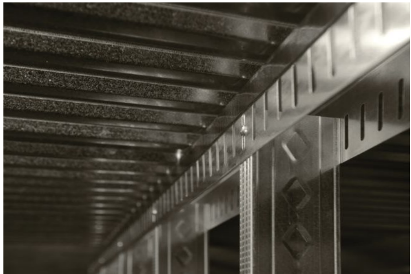
Fire Stop Deflection Track – BlazeFrame is a deflection track that includes a factory-installed intumescent strip affixed to steel profiles. When exposed to heat, the intumescent expands and forms a barrier to seal off joints (gap), preventing passage of flames, temperature pass through, and hot gases.
