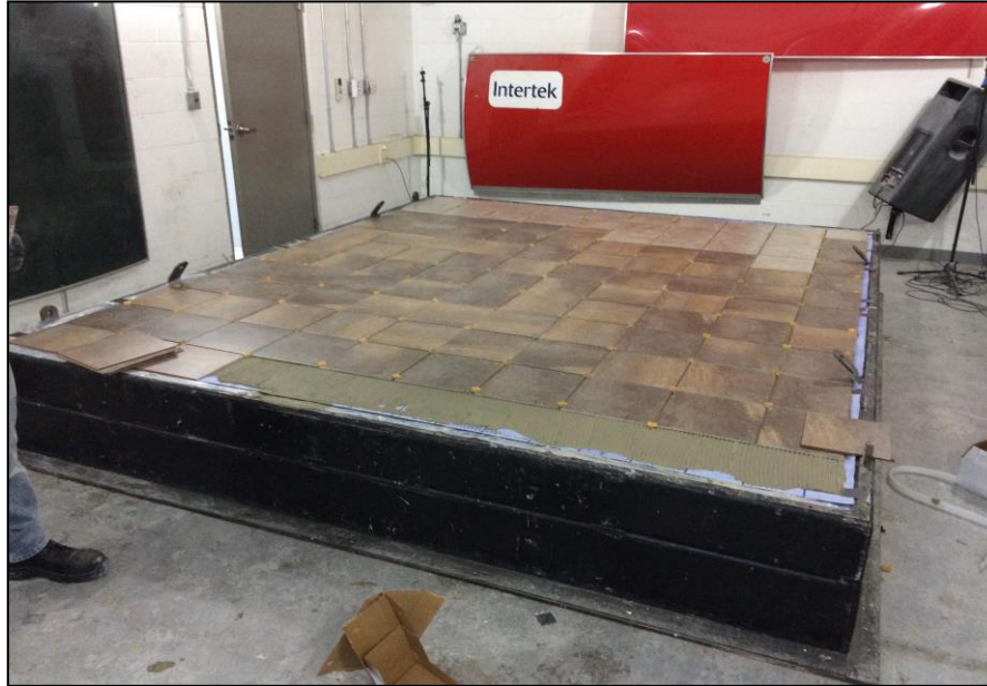
Photo No. 1 Construction of Test Specimen
