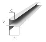
Designed to cover the raw edges of drywall and provide a 1/2" horizontal extension.
