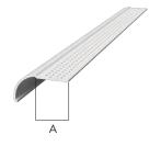
3/4" radius bullnose designed with a return leg that can be inserted into the channel of door and window jambs.
