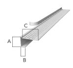
Designed to cover the raw edges of drywall when butting up to other materials such as masonry, glass, door frames, and window frames. Features a 5/16" removable leg that acts as a guide for the taping knife and a protective mask for joint compound application.
