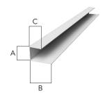
Designed to cover the raw edges of drywall under all window and door casings.
