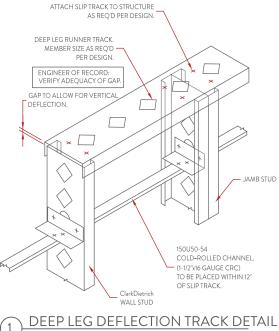
WITH LATERAL BRACING WITHIN 12" OF SLIP TRACK
