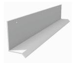
Designed to be used above window and door openings or at the floor line to assist with moving moisture away from the wall. May be used in combination with casing bead. Always caulk all intersections, butt joints, ends and corners at time of installation.
