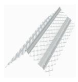
Clark Dietrich #2A galvanized corner bead, provides additional rigidity for reinforcing plaster corners. The #2A is an ideal choice for corners in high-traffic areas. Combination of expanded flanges and pronounced bead nose ensures effective corner alignment and efficient plaster keying from edge to nose.
