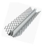
ClarkDietrich #30 Corner Master™ inside corner control joint is designed to provide stress relief at plaster wall inside corner intersections, by absorbing movement and controlling cracking. It has expanded flanges preformed at 90° for a flush fit at inside corners. Ground heights offered aid plaster keying and result in a clean, straight finish. Manufactured from galvanized steel for corrosion protection.
