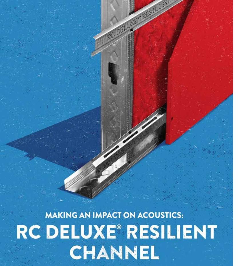
Resilient channels have long been a popular, cost - effective component of acoustical design strategies in commercial and multifamily construction projects. They function as decouplers, permitting the attachment of gypsum board to the framing members without any actual contact between the two components. This separation of the gypsum board from the studs impedes the transmission of airborne sound waves through the wall assembly by breaking their path.
