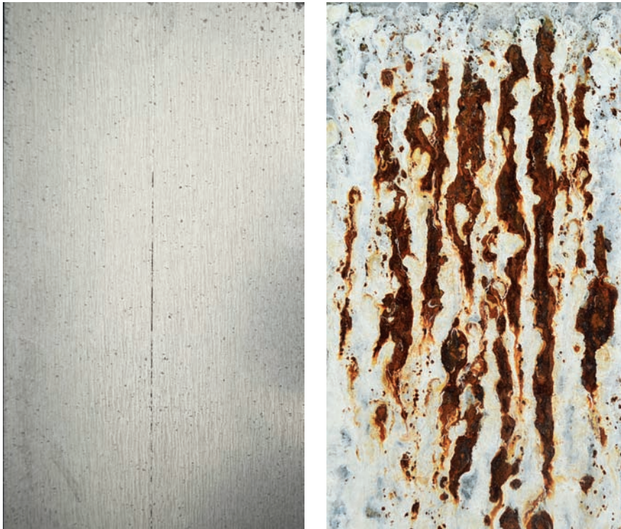
This side-by-side comparison shows the rust area of EQ-coated steel and G40 steel samples after 240 hours of salt spray testing.
