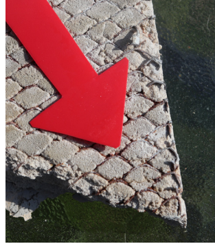
The galvanized metal lath eventually sacrifices the 3 mils of zinc coating to oxidize the carbon steel below.
