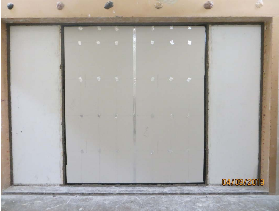
Figure 1 – Specimen mounted in test opening, as viewed from source room
