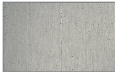
DiamondPlus SURFACE RUST AT 240 HOURS
