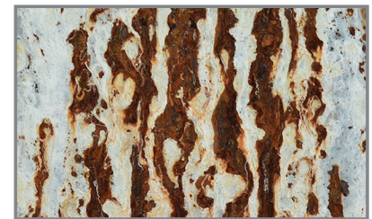
G40 SURFACE RUST AT 240 HOURS
